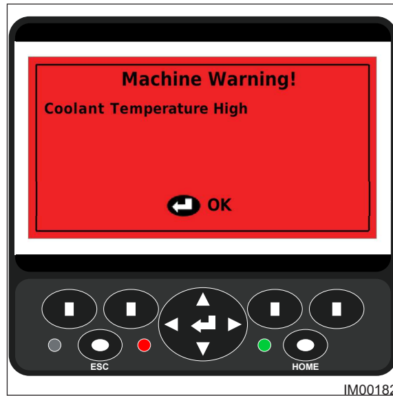
Fig: 4.13 - Machine Fault Pop-Up Screen
